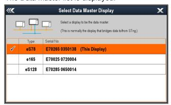
Select an MFD from the list that you want to designate as the Data master. This should be the MFD that is connected to the SeaTalkng® / NMEA 2000 network.
