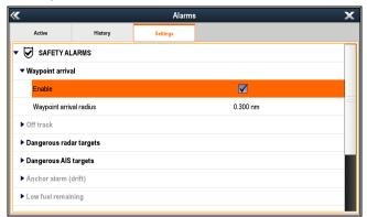
If the **Enable** box is ticked then the alarm is currently enabled.
