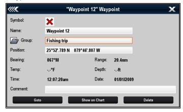
Selecting a text field displays the onscreen keyboard, which can be used to edit the details.
