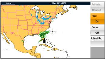
**Note:** You cannot display information (by moving the cursor over a symbol) when animation is running. The Range and Rotary controls do however remain operable provided the PAUSE option has not been selected. Ranging / panning will cause the animation to restart.
