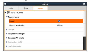
From the **Settings** tab you can enable and disable alarms and change alarm thresholds.
