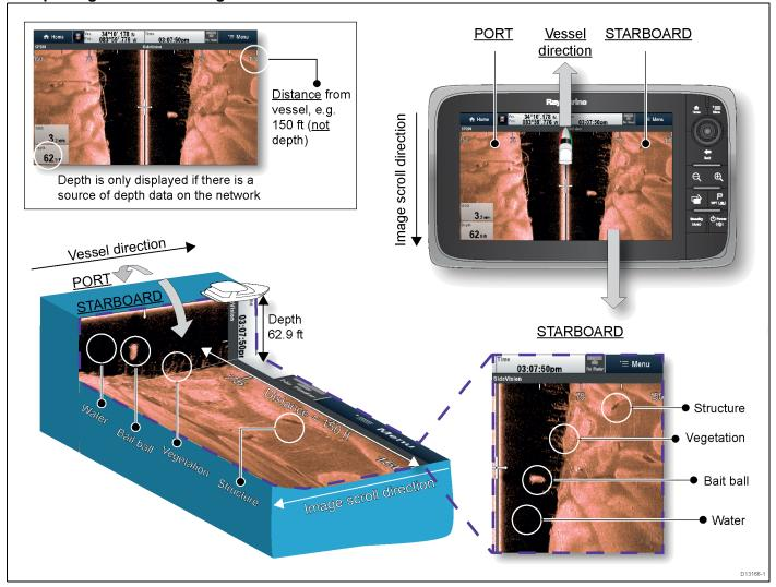
SideVision™ images are constructed line-by-line, similar to the way a television picture is composed of many horizontal lines. Each successive ping from the SideVision™ transducer adds a new line of image data to the top of your display. Each new line shows sonar returns from both the port and starboard sides of your vessel.
