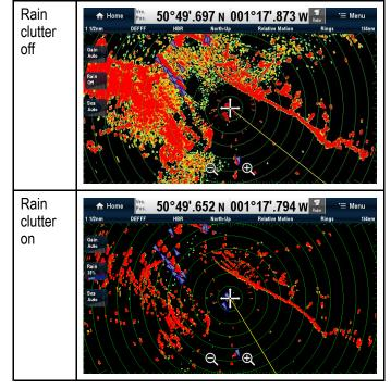
**Note:** Quantum uses pulse compression which filters out precipitation. However, you can identify/display precipitation using Quantum's **Weather** mode.
