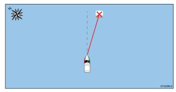
In **Head Up** mode, the Chart application displays the vessel's current Heading directly up. As the vessel Heading changes the vessel symbol remains fixed and the chart picture rotates accordingly. If Heading is not available then stable COG is used instead. If Heading or stable COG data is no longer present then the Orientation mode is suspended and the Chart application will display 0 degrees directly up if there is no active navigation or Course Up if there is active navigation.
