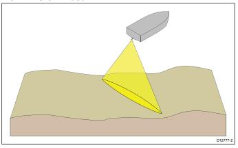
**DownVision™** is effective at lower vessel speeds. In deeper waters the CHIRP bandwidth is automatically optimized to improve bottom lock and the detection of moving objects (e.g. fish) in the wider water column.
