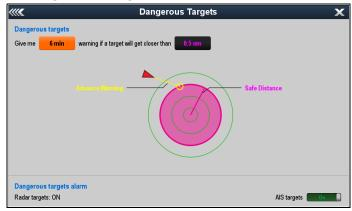
E.g.: With **Time to Safe Distance** set to 6 minutes and the **Safe Distance** set to 0.5Nm, AIS targets will turn red and start to flash if they will reach the Safe Distance within the next 6 minutes.
