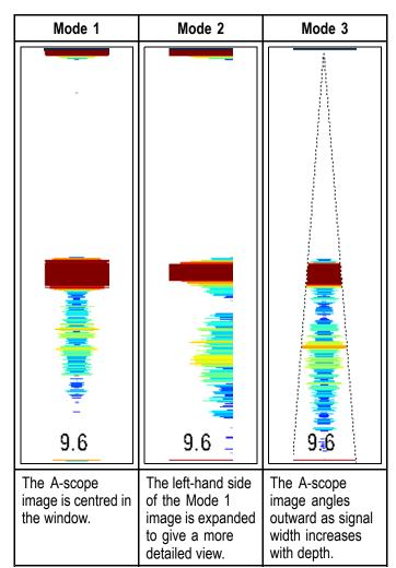
The numbers displayed at the bottom when in A-Scope mode indicate the approximate diameter (in selected depth units) of the conical beam's coverage of the bottom.
