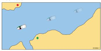
When the motion mode is set to True Motion, the chart is fixed and the vessel moves in true perspective to fixed landmasses on-screen. As the vessel's position approaches the edge of the screen, the chart picture is automatically reset to reveal the area ahead of the vessel.
