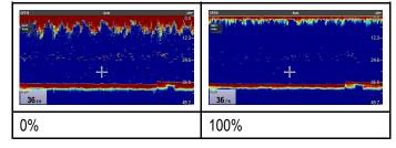
The Surface filter can be set to automatic or can be adjusted manually. In manual:
