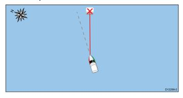
In **Course Up** mode, during active navigation, the Chart application displays the vessel's current destination waypoint directly up. When the destination waypoint changes the chart picture rotates accordingly. The reference used for Course Up depends upon the information available at a given time. The system always prioritizes this information in the following order:
