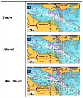
The level of detail shown on-screen is also affected by the cartography **Chart detail** settings. Refer to **Chart detail** for information.
