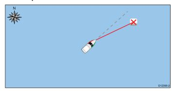
In North Up mode, the Chart Orientation is fixed with true north pointing up this is the (usual orientation of nautical charts). As your heading changes the vessel symbol rotates accordingly. This is the default orientation for the Chart application.
