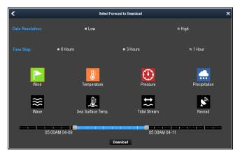
Sea Surface Temperature, Tidal Stream and Nexrad data must be downloaded individually, Wind, Temperature, Pressure, Precipitation and Wave data can be downloaded individually or combined together.
