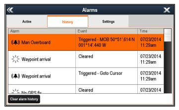
The Alarm History tab provides details of alarms and the date and time that they were triggered and cleared / acknowledged. The Alarm history can display up to 1,000 alarm events and displays them sorted by time.
