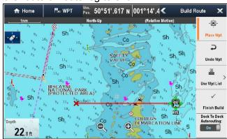
The system will try to automatically calculate the shortest safe route between the 2 points.
