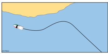
Each track can contain up to 10,000 track points, when the track limit is reached the track is saved and a new track is started automatically. Up to 15 tracks can be saved and a 16th track may be active (currently recording), if the track limit is reached for the 16th track then the user will be prompted to delete a current track or stop recording, otherwise the earliest track points will be overwritten with the new track points.
