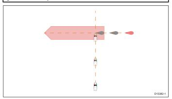
In the example above the vessel's COG will cross with the target's COG within the Interception zone, which could cause a collision. You should alter course and / or speed to avoid the potential collision.
