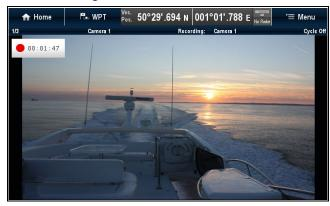
Whilst the camera application is recording you can use your multifunction display as normal e.g. view a different camera feed, go back to the Homescreen, or open a different application. The selected feed will continue to record until stopped or until the memory of the selected location is full.
