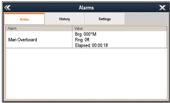
The Active Alarm tab lists all currently active alarms. Alarms are removed from the list when:
