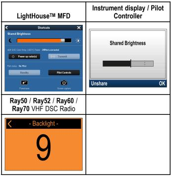
Multiple brightness groups can be configured. These groups could be used to reflect the physical location of units on your vessel. For example, the units at your helm can be set to one group, and the units on the flybridge can be set to a different group.
