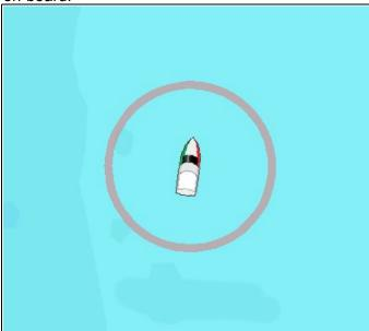
The fuel range ring can be displayed graphically in the chart application and indicates an estimated range that can be reached with the:
