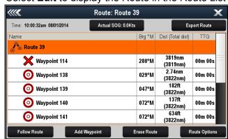
You can further customize the route from the route list. Reviewing the route list is not an adequate method of checking a route, please refer to Reviewing an automatically generated route for details on how to check a route.
