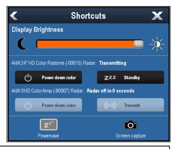
**Note:** If you have 2 Radar scanners connected; options for each Radar scanner will be shown.
