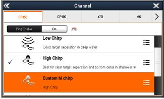
8. Select the new channel to display it in the Sonar application pane.
