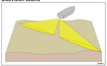
**SideVision™** is effective at lower vessel speeds. The wide, thin beams produce clear target returns. As your vessel moves forward, subsequent returns build up to provide an image of the sea floor on each side of your vessel.
