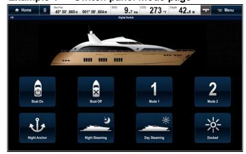
If configured a Mode page provides controls to switch between pre-configured modes.
